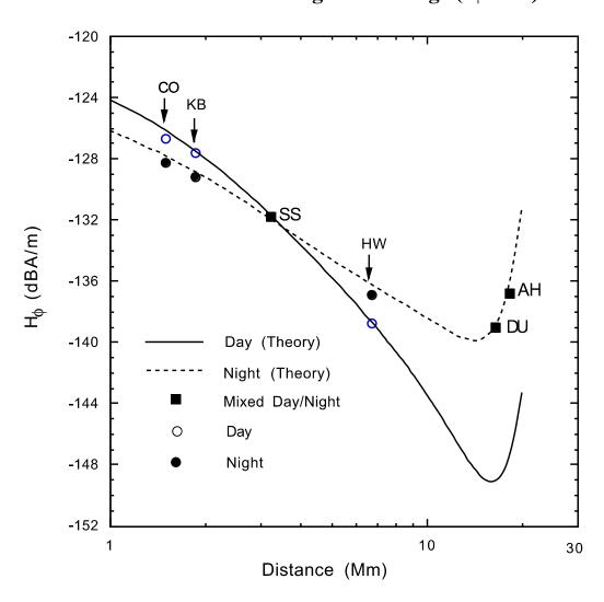
Figure 2. Curves showing measured and predicted values of the KPTF 82 Hz field strengths. The two curves show theoretically-predicted values for all-day and all-night paths over global ranges and the measured field strengths at Søndrestrømfjord (SS), Dunedin (DU), and Arrival Heights (AH) are shown as three labelled points. January WTF/MTF 76 Hz field strengths in Connecticut (CO), Hawaii (HW), and at King's Bay, Georgia (KB) are also shown for comparison.
