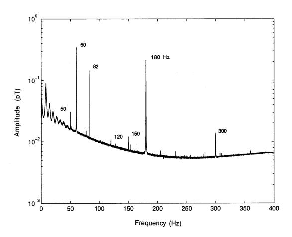
**Figure 1**. Average amplitude spectrum of the lower-ELF radio noise at Søndre-strømfjord, Greenland, during January, 1990. The average spectrum is computed from the 1185 one-minute synoptic recordings taken twice per hour that contained 82 Hz transmissions; the overall total possible number of these one-minute recordings during January is 1488.
