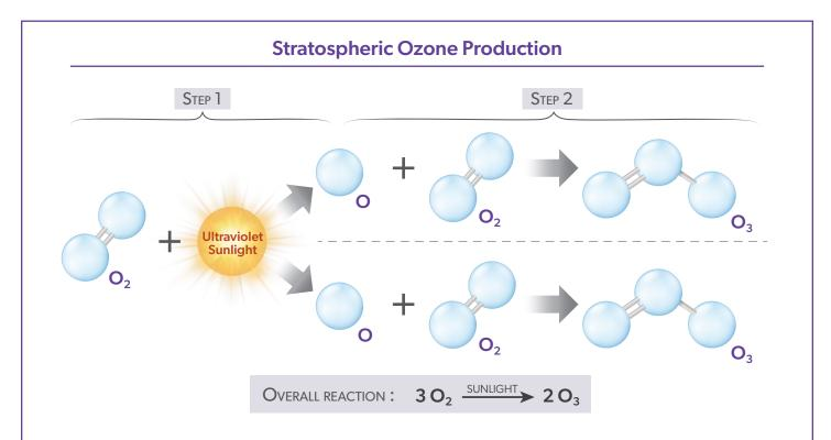
Figure Q1-3. Stratospheric ozone production. Ozone is produced naturally in the stratosphere by a two-step reaction process. In the first step, solar ultraviolet radiation (sunlight) breaks apart an oxygen molecule to form two separate oxygen atoms. In the second step, each oxygen atom collides with another oxygen molecule and forms an ozone molecule in a binding reaction. In the overall process, three oxygen molecules plus sunlight react to form two ozone molecules.
