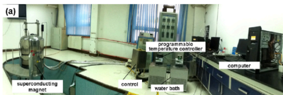
Figure 6. Overall configuration of the instruments with a large-gradient high-field magnet. (a) photograph of the system and (b) a schematic illustration of the system. Four special positions in the magnet bore (simulated 0 g, 1 g, 1.56 g and 1.96 g) and a control were utilized for placing the samples
